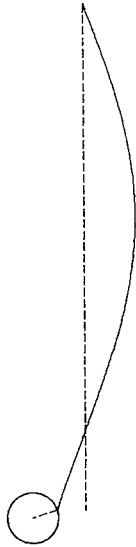
Fig. 3 Graphic representation of the modal ratio between skip-rope and satellite pendulous motion amplitude.
